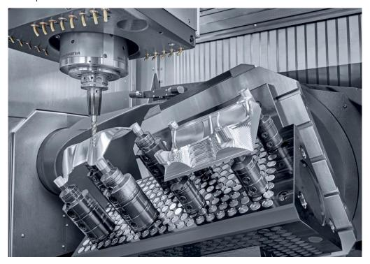
The DMC 65 monoBLOCK 2. Generation and DMC 75 monoBLOCK 2. Generation enables efficient 5-axis simultaneous machining of complex workpieces up to  $\emptyset$  630 x 500 mm and 600 kg.
